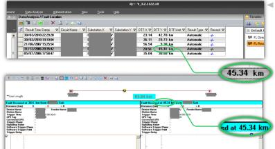
IiQ<sup>+</sup> software and traveling wave distance to fault calculation from end X
